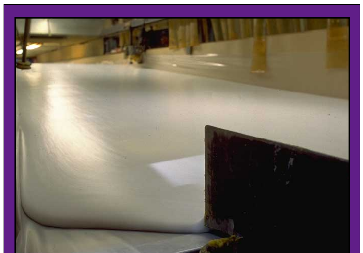
Viscoelastic foam can be manufactured using conventional flexible polyurethane foam slabstock and molding processing equipment.
