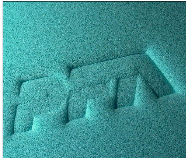
Viscoelastic foam is characterized by slow recovery after compression. Its ability to closely contour to shapes allows surface pressure to be distributed over a wide area.
