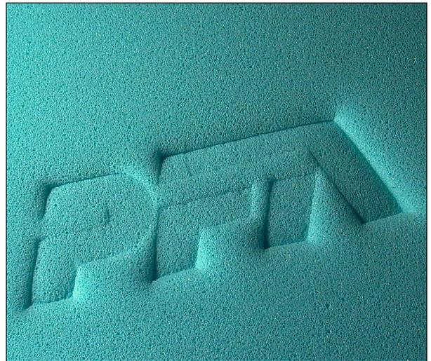
Viscoelastic foam is characterized by slow recovery after compression. Its ability to closely contour to shapes allows surface pressure to be distributed over a wide area.
