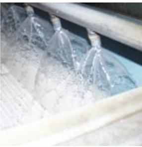
**3. Washing:** Upon completion of the molding process, the latex foam is placed on a conveyor belt and put through a large washer to rinse and remove proteins, soap residue and improve product durability through a five-stage wash/squeeze cycle process.
