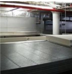
**4. Drying:** The mattress core or pillow is then transported by conveyor belt to a dryer. The core or pillow bun is slowly run on another conveyor belt through the dryer, which evaporates the liquids to finalize the curing process.
