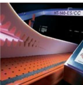
**6. Fabrication:** Cores are transported from the core bank to the fabrication area on a just-in-time basis. Here, the core is cut and constructed to the appropriate size. When larger core sizes and heights are needed, smaller cores are affixed with environmentally sound, water-soluble latex adhesive.
